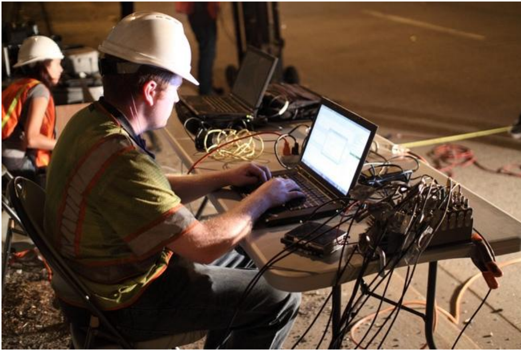
Figure 3. National Instrument cRIO data acquisition system used for impact testing campaigns on bridge
